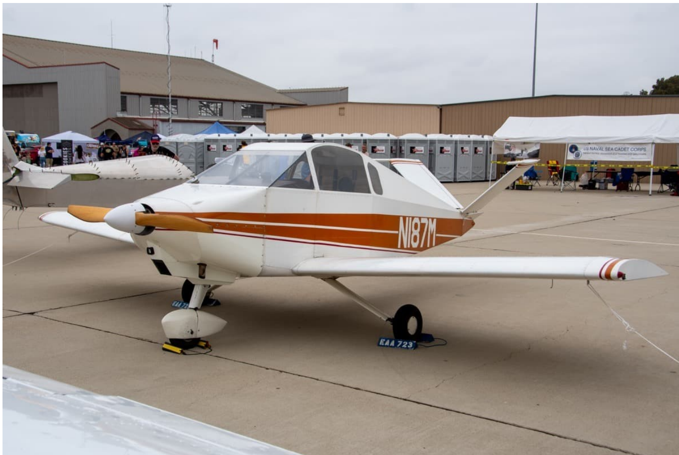
A Davis DA-2A homebuilt with a flat-sided "box" fuselage and angular appearance, designed intentionally for ease of construction. First flown in 1966, it won several awards at Oshkosh that year, including "most outstanding design."
